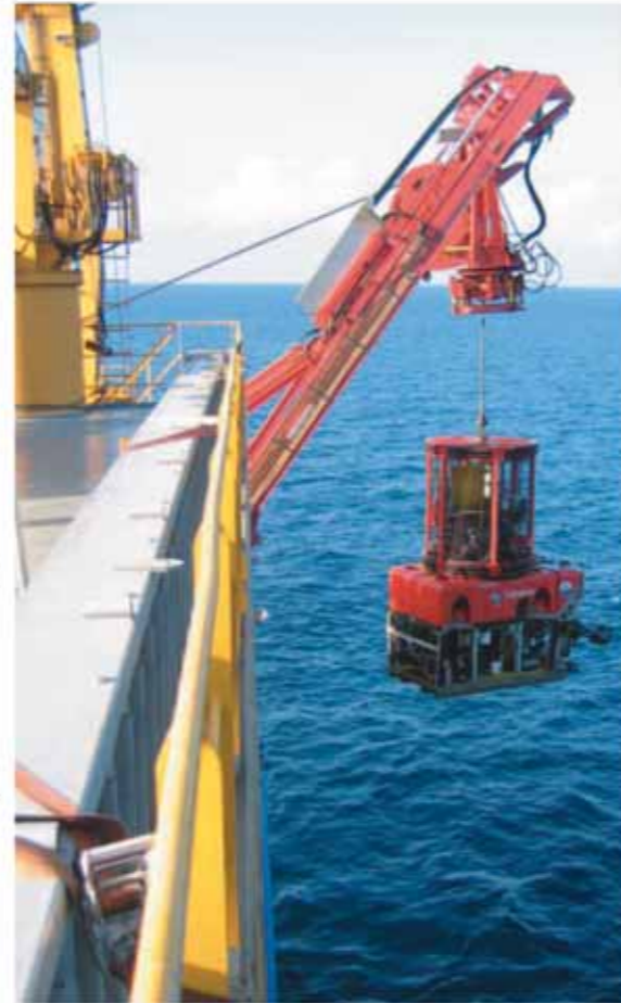
Figure 1. The remotely operated vehicle is brought onboard the cable-deploying vessel after laying cable on the seafloor. (Photo courtesy of Multiwave Geophysical)
